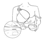
Connect the pump by putting the cannula into the marked opening on the breast form. Open the valve inlet by gently squeezing the thumb and index finger together. Make sure you insert the cannula completely into the valve.
